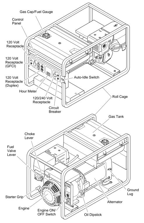
Figure 1 - Portable Generator (Model PGH7500IE Shown)
